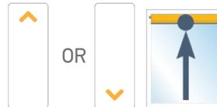
**Step 4:** **PRESS & HOLD** the **MY/STOP** button until the shade jogs, then release. Check the new limit.
