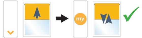
**Step 3:** Bring the shade to your desired upper limit. **PRESS & HOLD** both the **MY/STOP and DOWN** buttons until the shade begins to move down, then release. Stop the shade at the desired lower limit, adjust by pressing the **UP or DOWN** buttons.
