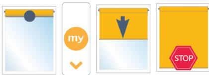
**Step 4:** **PRESS & HOLD** the **UP and MY/STOP** buttons until the shade begins to move up. The shade will stop at the original upper limit. Adjust if necessary.
