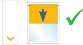
If the shade raises instead of closing, change the direction - **PRESS & HOLD** the **MY/STOP** button until the shade jogs. Confirm correct direction of operation before proceeding.
